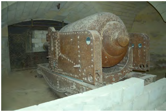
Fig. 19: The British guns are used in well-walled casemates of Fort Delimara to protect against the weather.
